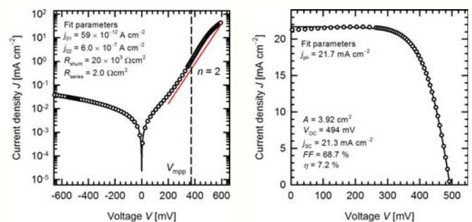
In-house measured dark (circles) and fitted (line)  $J$ - $V$  curve of the MacPSi cell. The red line is a plot for  $n = 2$ .
