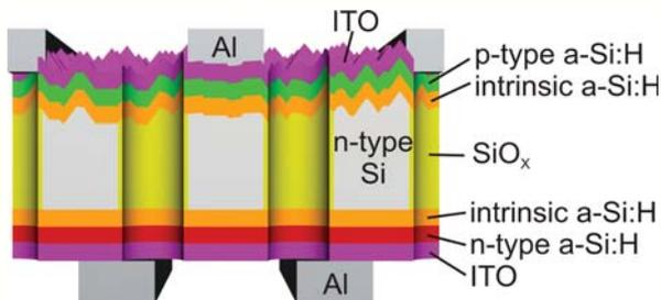
Schematics of the macroporous silicon solar cell (not to scale).
