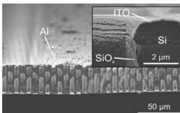
Cross section of an identically processed MacPSi cell with an Al finger. The inset shows the oxide layer on the pore walls as well as the ITO layer at the surface.
