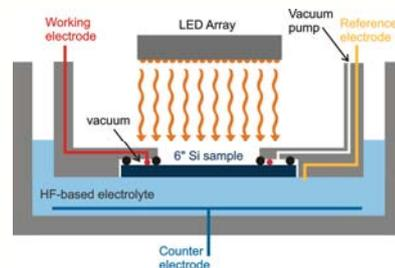
Schematic of the electrochemical etching setup with rear-side illumination
