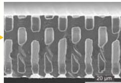
Cross section of a detached and free-standing ( $33 \pm 2$ )  $\mu\text{m}$  thick macroporous Si absorber layer.
