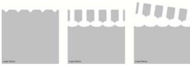
Illustration of formation and separation of a macroporous Si layer from a substrate wafer. Finally, the substrate is cleaned for re-use.
